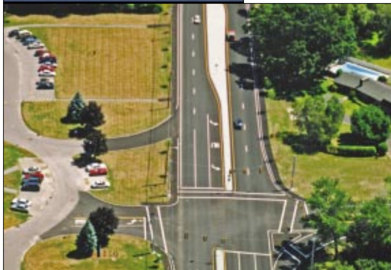
River Road in Andover, Mass., is an example of access management techniques applied to local highways. These techniques preserve the safety, function and capacity of the corridor for cars, bicycles, and pedestrians.
