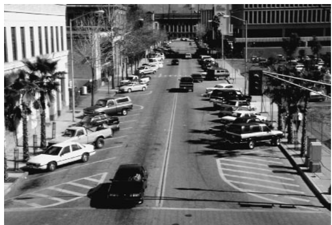
Figures 2-3 and 2-4. European experience with traffic calming is very extensive; this town is one of hundreds in Denmark that have redesigned their residential and commercial streets to make them more pedestrian-friendly (Figure 2-3). In the United States, cities like San Bernardino, CA, have begun traffic calming efforts of their own, in this example by introducing diagonal parking (Figure 2-4). (Credit: Project for Public Spaces, Inc.)
